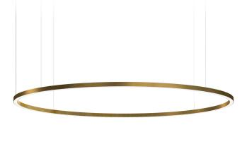
Suspension lighting fixture for interiors, with direct light emission. Bended extruded aluminium structure in white, black or mat brass polyacrylic paint. Extruded polycarbonate diffuser with opaline finish. Suspension kit with griplocks and 5m (196,9") long steel cables. 5m (196,9") long power cable in transparent PVC. Power canopy with pickled sheet metal ceiling bracket and covering in white polyacrylic paint.
